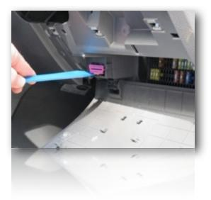
2. Remove the existing OBD port from its mounting place using a trim removal kit and tools.
