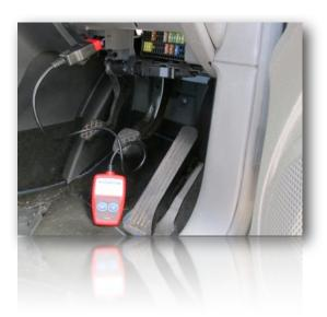
9. Check for communication with vehicle system used for Key Programming.
