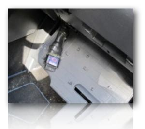
6. Fit the new cable into the existing mounting position of the original OBD port.
